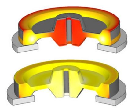
The upper image shows the distortion that occurs during an intermediate machining pass, while the lower image displays the distortion in the final pass.
