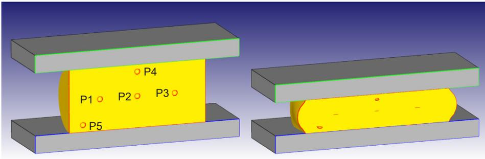
Contrast that with the RVE approach. The first step in the RVE approach is to run a component-level simulation without microscale features. This runs relatively quickly due to the moderate model size. Point-tracking provides the thermo-mechanical history that will be used as an input to subsequent RVE models.
