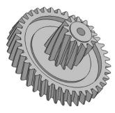
It is common for such a gear to spin during the peening process, with the spray nozzle moving up and down while firing the shot.
