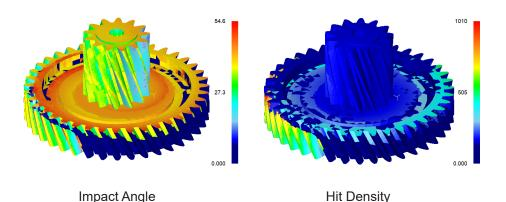
The shot peening conditions influence the final residual stress state of the part, as shown below. Well peened regions are in a state of residual compression (green) while unpeened regions are essentially stress-free (white). With this nonuniformity identified, DEFORM could then be used to evaluate alternate process designs. These simulation studies will allow users improve coverage and make residual stresses more homogeneous.
