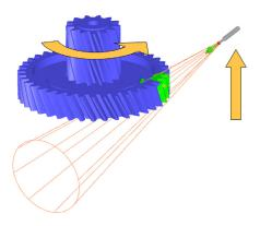
The shot peening of this gear can be modeled by following an easy-to-use, wizard-based template. The user is guided through the workflow to import CAD models and mesh the gear geometry. Objects that might impede the shot hitting the gear, providing a shadowing effect, could also be added.
