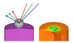
At a larger scale, process parameters such as workpiece rotation, the shot spray zone and movement are considered. All of this information is utilized to predict residual stress response and shot peening coverage at the part level.
