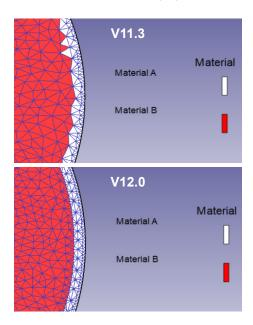
New local remeshing methods allow users to remesh a specific portion of the workpiece, rather than the entire part. State variables and geometry outside of the local zone thus remain unmodified. This benefits applications that require fine detail but involve many remeshes, such as in machining (bottom). Here, a user-defined window, which follows a cutting tool, defines the remeshing zone.
