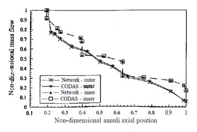
Figure 5: Annular combustor 2: Comparison between network methodand CODAS results for non-dimensional mass flow vs. non-dimensional annuli axial position.
