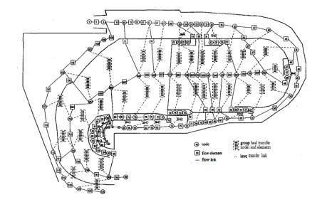
Figure 2: Network diagram for reverse flow combustor
