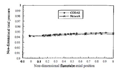
Figure 6: Annular combustor 2: Comparison between network methodand CODAS results for non-dimensional total pressure vs. nondimensional flame tube axial position.
