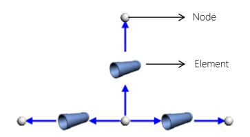
Figure 1: Network showing elements and nodes.
