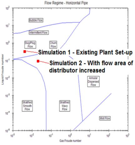
"The resultant pressure drop caused more flashing across the control valve and moved the flow regime away from the slug flow area"
