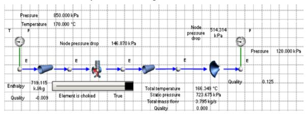
Figure 2: Flownex simulation of the deaerator system.
