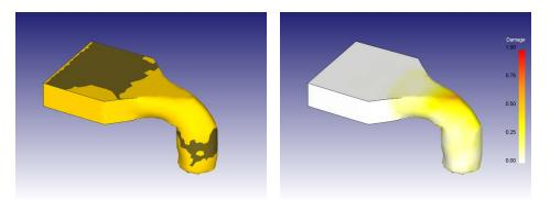
Physical product testing of the prototype later revealed that more die fill was desirable. Toolmakers again used simulation and shop trials to further optimize the design. A fourth forming operation was subsequently added to the process. High-volume tooling was manufactured when the job was launched into production.
