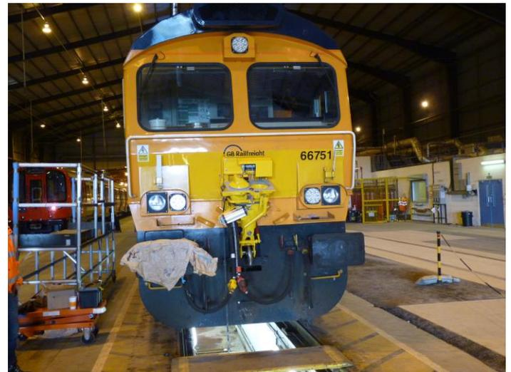
*Class 66 loco with coupler support frame (Courtesy: ESG Rail)*
