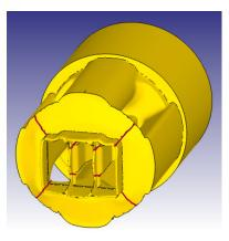
Ongoing developments in mesh generation allow the creation of a structured mesh (shown below) that is optimized for extrusion, with excellent feature definintion.
