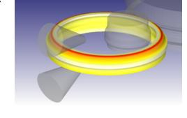
and contact algorithms are optimized for ring rolling. The result is an accurate solution, without artificial constraints on the rotation axis.
